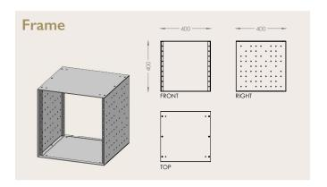
The frame is produced of 1,5 mm steel plate, powder coated in standard colors or according to an interior plan. The frame is open in two sides which can be used for a door, perforated steel
