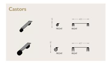
Castors are available in two sizes depending on the size of the BRICKS composition. Castors are also available with brakes.
