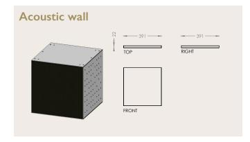
The BRICKS locker units can have an upholstered back panel for noise absorbtion, or just for nice decoration. Any fabric from an interior plan can be used.
