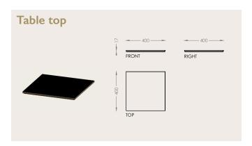
The top of the Bricks compositions can have a table top made of veneer or laminate. Other materials by request.
